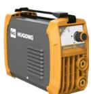
KEY FEATURES ▶ TIG/Stick output 10–160 A; duty cycle 60 % @ 160 A ▶ HF start TIG, step-less amperage control ▶ 230 V single-phase IGBT inverter, generator safe Weight 6.8 kg: hotstart & fan cooling
